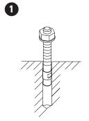
BORE 4 HOLES IN KEEPING WITH THE DIAMETER OF THE PLUGS AND THE PASSAGE
